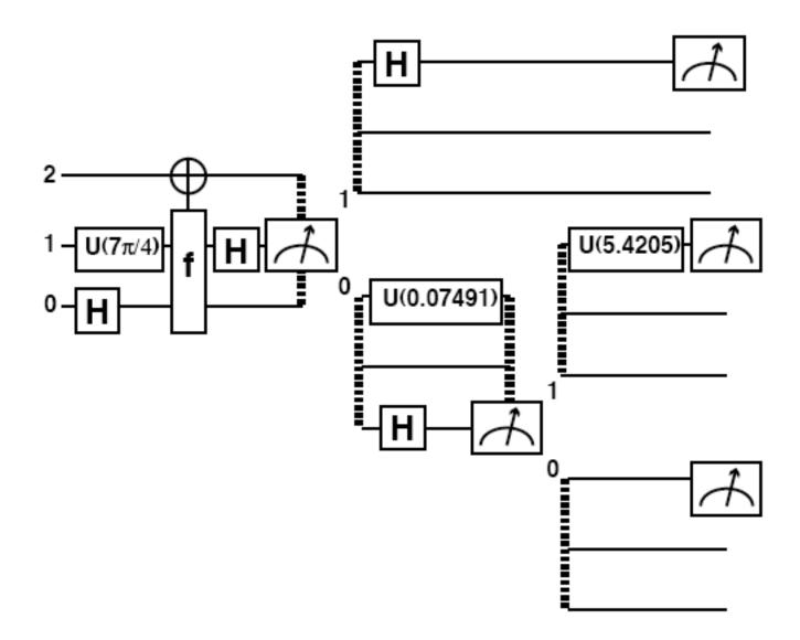
*Figure 8.11.* A gate array diagram for an evolved solution to the AND/OR oracle problem. The gate marked "f" is the oracle. The sub-diagrams on the right represent the possible execution paths following the intermediate measurements.
