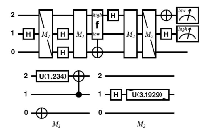
Figure 8.7. A gate array diagram for an evolved version of Grover's database search algorithm for a 4-item database. The full gate array is shown at the top, with  $M_1$  and  $M_2$  standing for the smaller gate arrays shown at the bottom. A diagonal line through a gate symbol indicates that the matrix for the gate is transposed. The "f" gate is the oracle.
