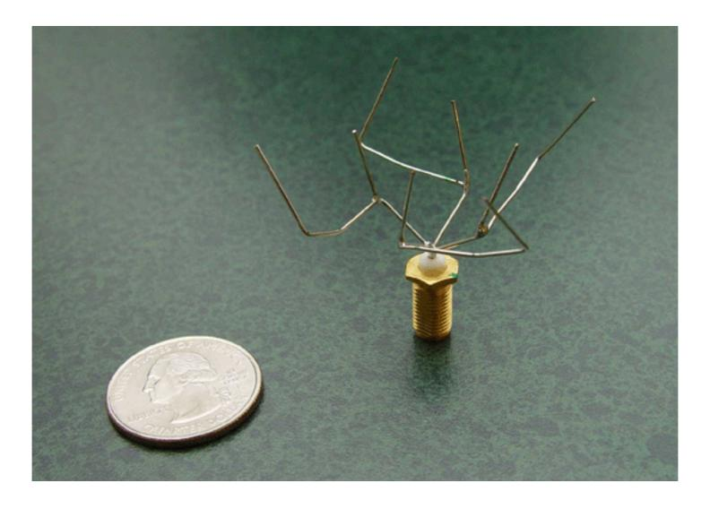
An Evolved Antenna for Deployment on NASA's Space Technology 5 Mission
